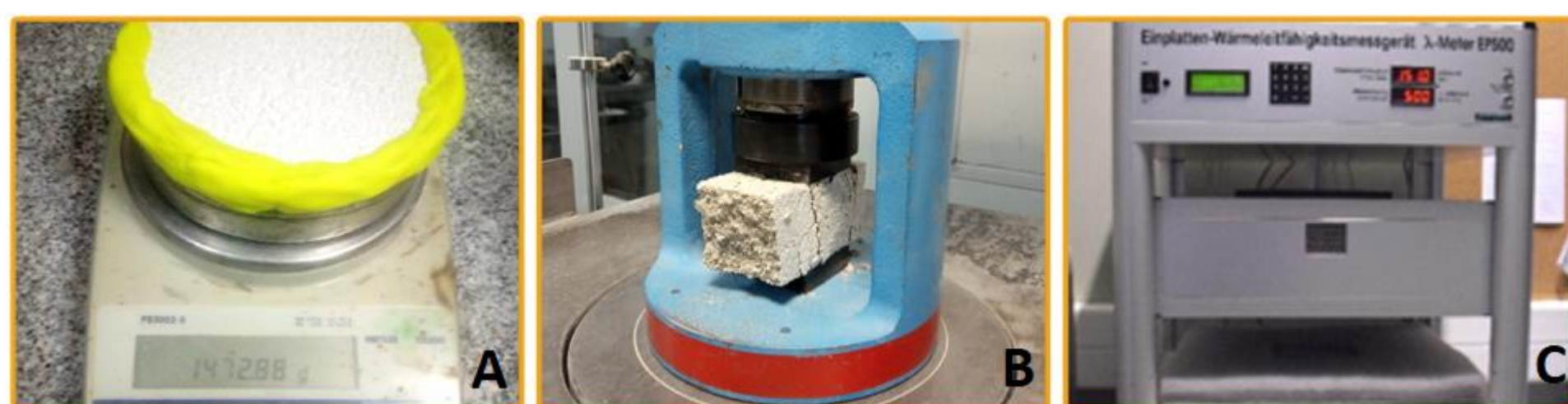
Figure 2: A - test specimen for water vapor permeability; B - test specimen for compressive strenght; C - thermal conductivity test
